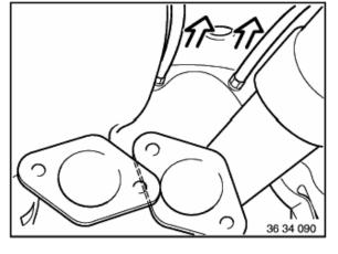
Remove final muffler (not necessary with compact), refer to Gr. 18
