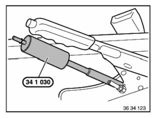
Loosen lock nut using special tool 34 1 030 and unscrew together with adjusting nut.
